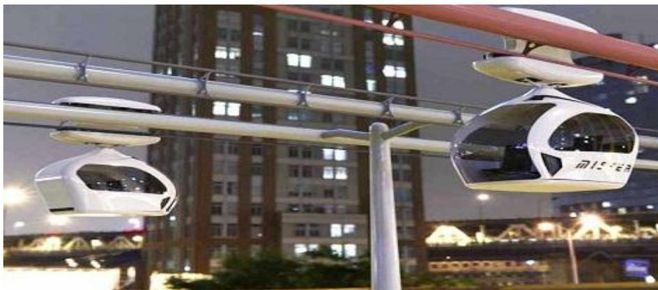
⇒ Small automated vehicles/podcars/cable cars which carry a small number of passengers. The ropeway-like system runs on electricity and driverless pods and comes down at designated stations, thus removing the traffic burden from crowded roads.
