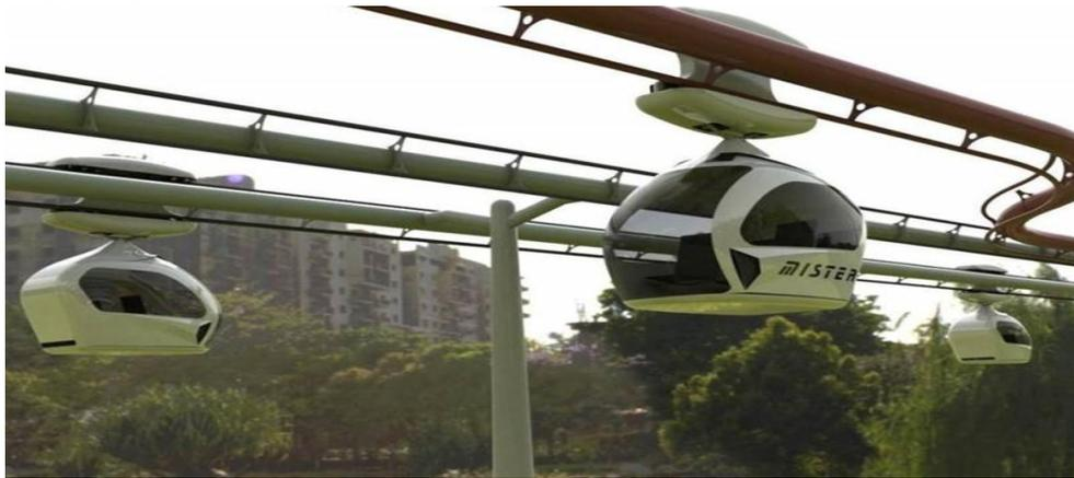
⇒ Fully automatic, driverless small pods travel independently suspended over an overhead network which is usually 5-10 meters above the ground.
